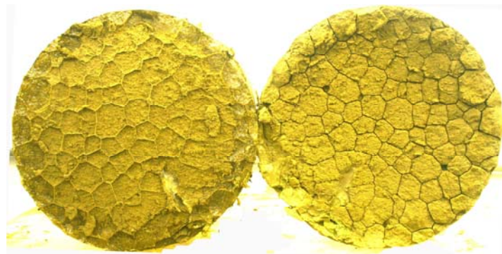
Figure 5. Cross sections of the sample at the end of test No. 1. The section on the left is the frozen sample, and the section on the right the unfrozen sample.
